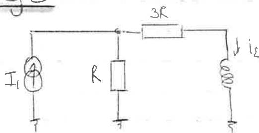
$$\textcircled{1} \quad Z_R = 3R \quad \& \quad Z_L = j\omega L \quad \& \text{ serie} \\ \rightarrow Z_{\text{tot}} = 3R + j\omega L$$
